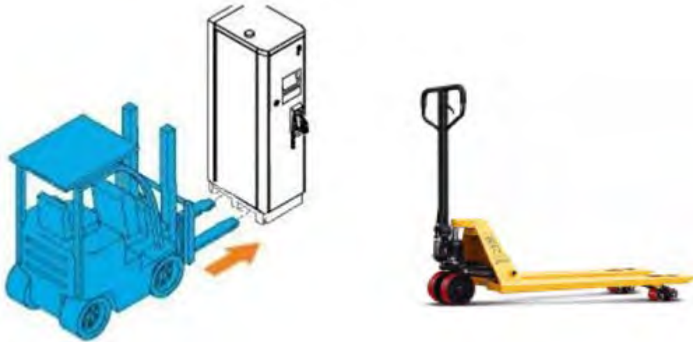
Figure 4-3 Move the EV Charger with forklift
