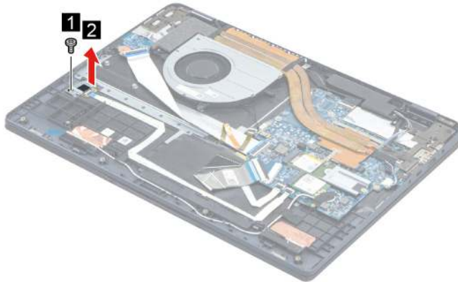
Figure 62. Remove the fingerprint board bracket
