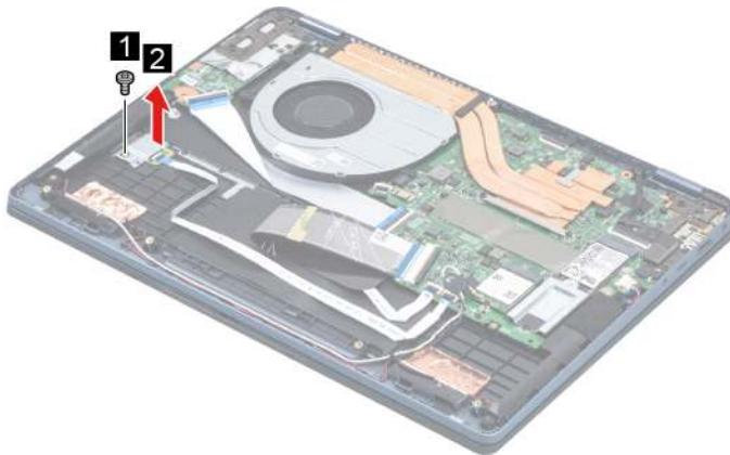
Figure 19. Remove the fingerprint board bracket
