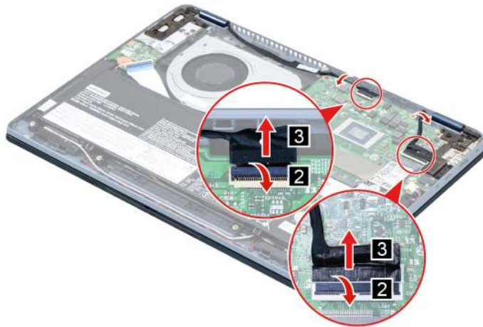
Figure 34. Disconnect cables connected to the system board
