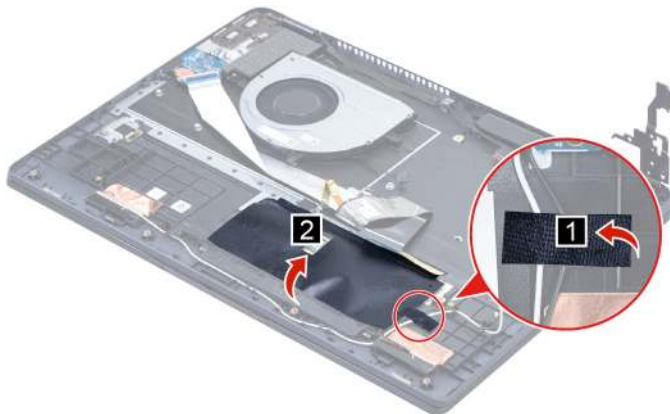
Figure 70. Remove the two pieces of tape
