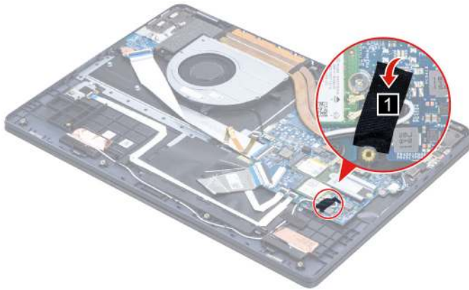
Figure 55. Peel off the pieces of tape
