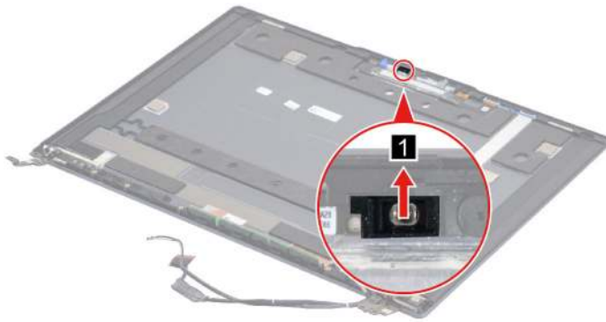
Figure 46. Remove the ToF rubber
