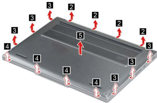
Figure 7. Remove the lower case
