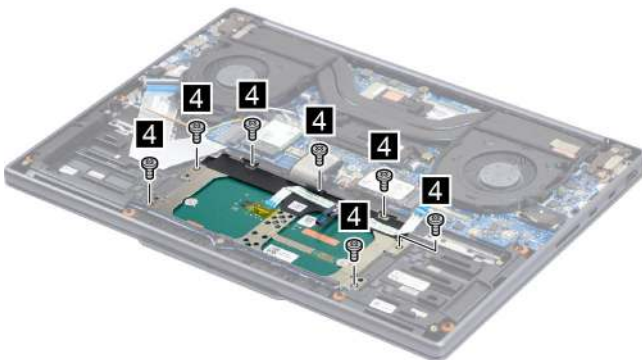
Figure 18. Remove seven screws
