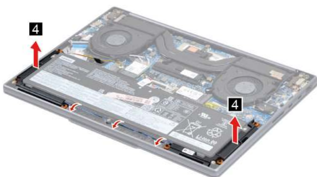
Figure 16. Remove the speakers
