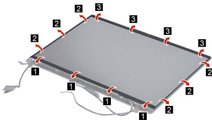
Figure 32. Remove the LCD bezel
