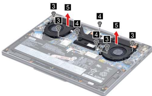
Figure 22. Remove the thermal module (Intel models)
