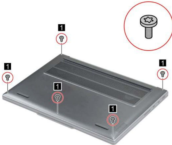
Figure 6. Remove five screws
