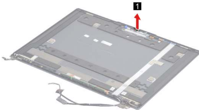
Figure 47. Remove the camera shutter
