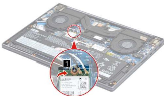
Figure 12. Remove the Wi-Fi card mylar
