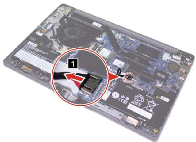
Figure 48. Disconnect the battery pack cable
