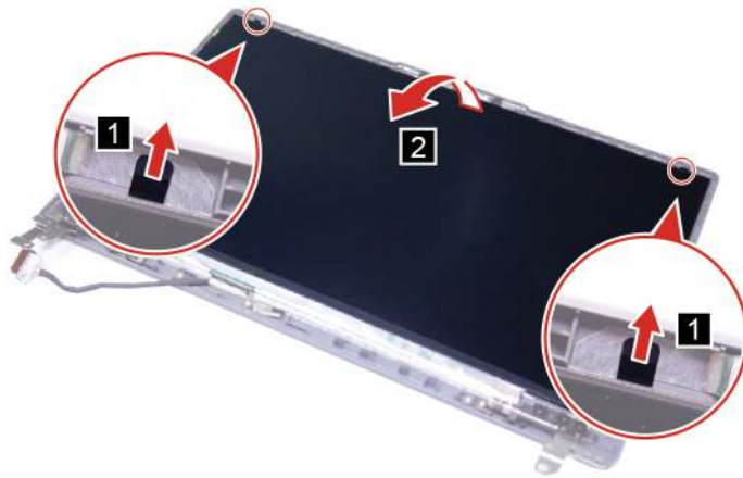
Figure 55. Remove the LCD panel
