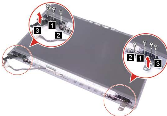
Figure 57. Remove eight screws and hinges
