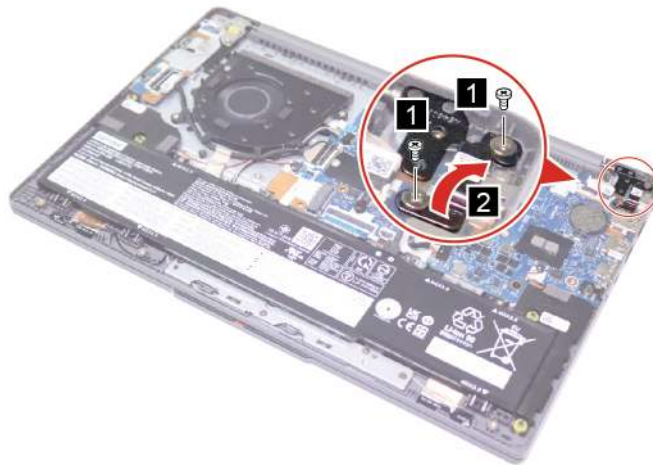
Figure 42. Remove two screws and lift the right hinge
