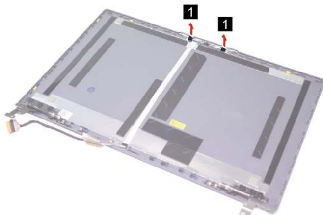
Figure 60. Remove the microphone rubbers
