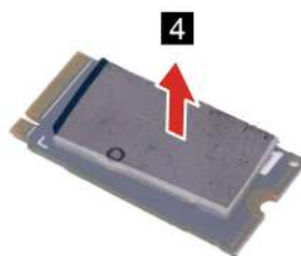
Figure 11. Remove the 2242 solid-state drive thermal pad
