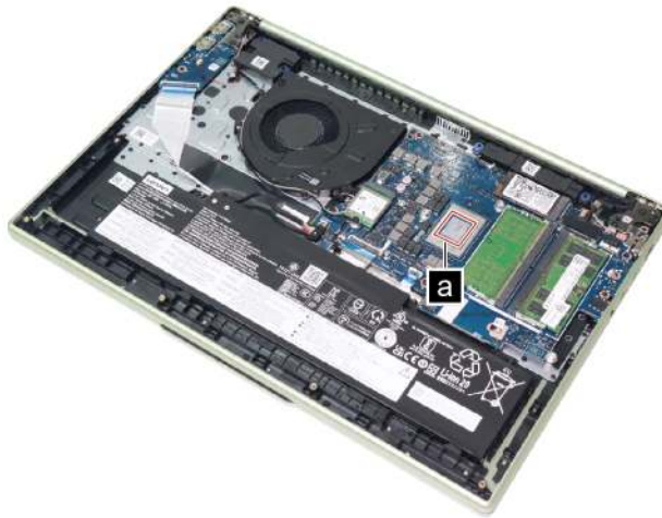
Figure 17. Area on the system board where thermal interface materials are applied (for AMD models)
