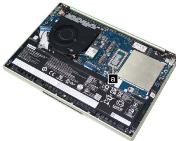
Figure 16. Area on the system board where thermal interface materials are applied (for Intel models)
