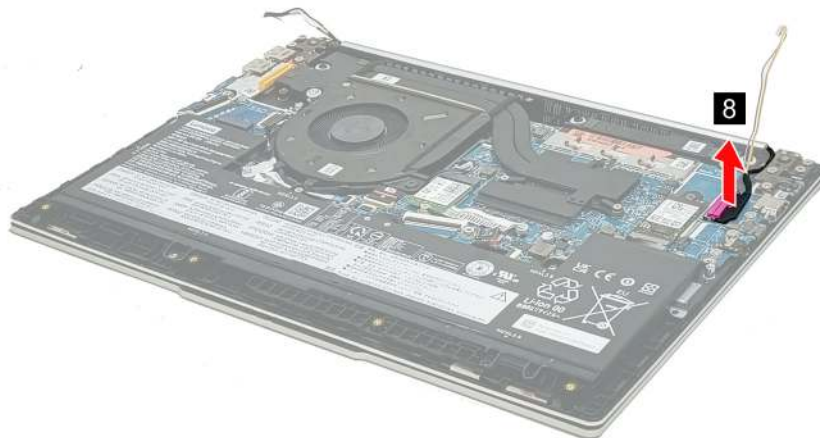
Figure 32. Disconnect the EDP cable from the system board
