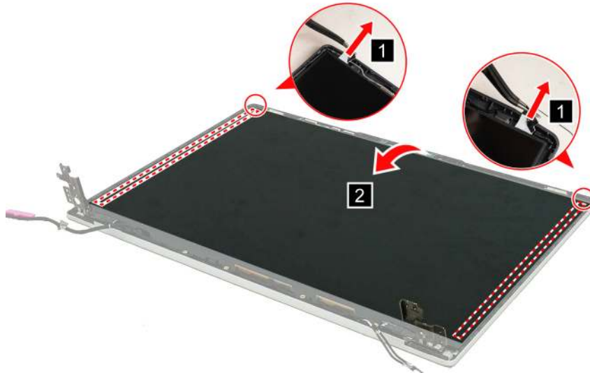
Figure 38. Pull out two pieces of removable tape and turn over the LCD panel
