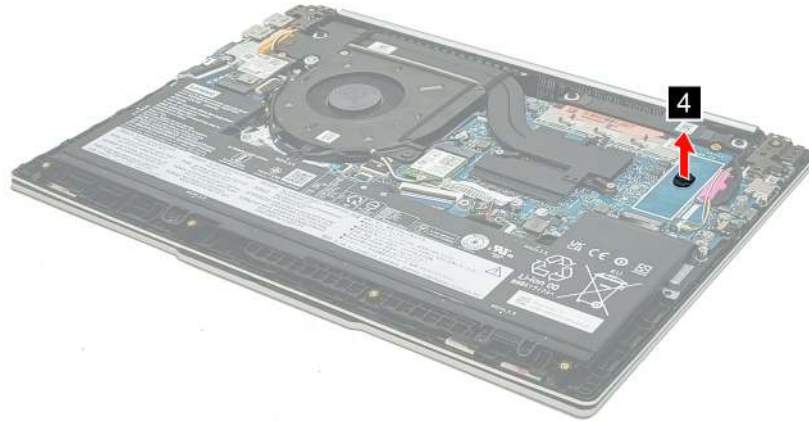
Figure 10. Remove the 2242 SSD holder
