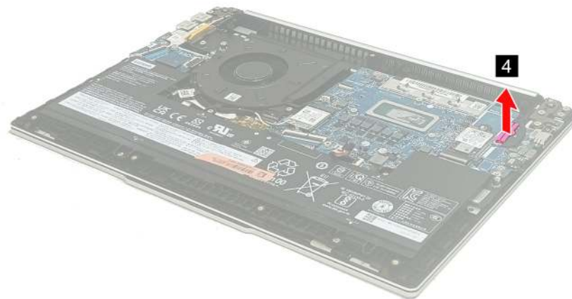
Figure 23. Remove the speaker cable rubber
