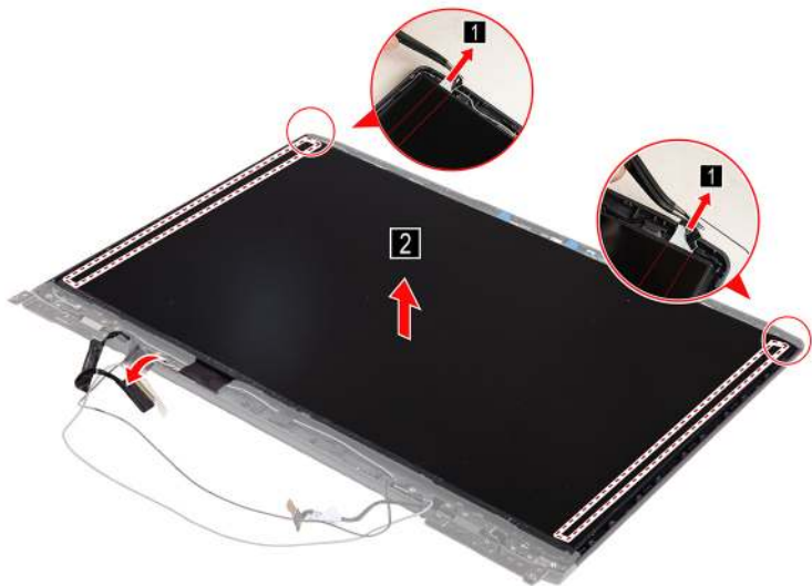
Figure 32. Remove the two pieces of removable tape with tweezers
