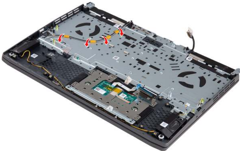
Figure 26. Release the antenna cable
