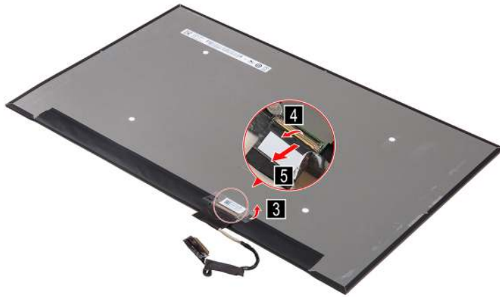
Figure 33. Disconnect the EDP cable
