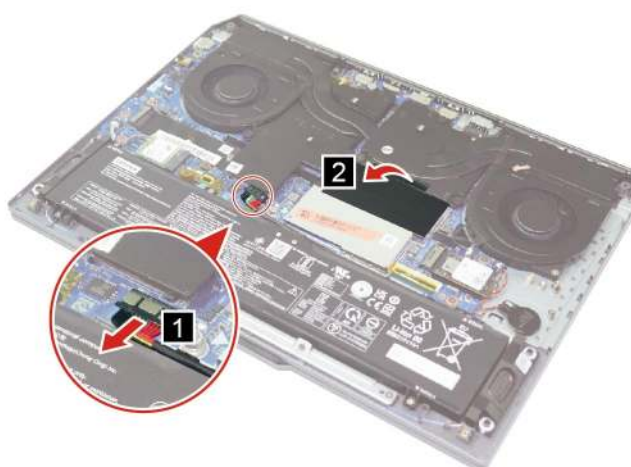
Figure 15. Disconnect the battery pack cable and peel back the mylar
