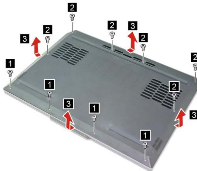
Figure 5. Remove ten screws and the lower case
