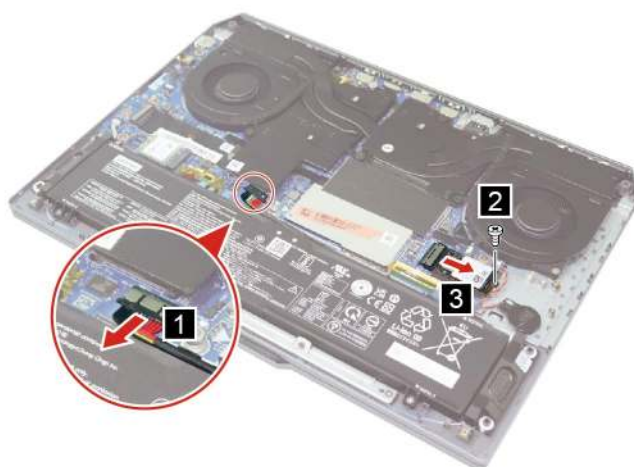
Figure 12. Disconnect the battery pack cable, remove one screw, and remove the 2242 solid-state drive
