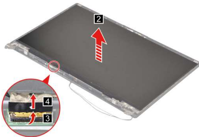
Figure 72. Lift the LCD panel and then disconnect the EDP cable from the LCD panel
