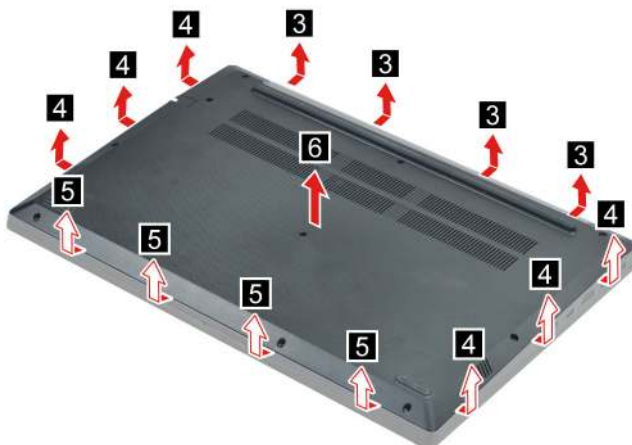
Figure 42. Pry up the latches and remove the lower case
