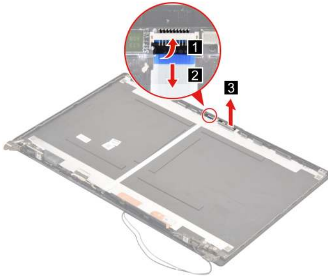
Figure 75. Disconnect the EDP cable from the camera board and then remove the camera
