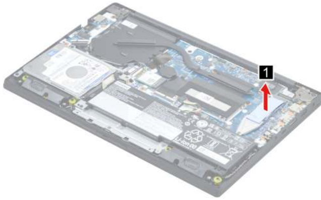
Figure 12. Remove the SSD thermal pad
