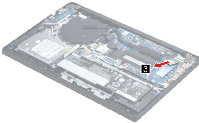
Figure 50. Remove the SSD by pulling it away from the slot
