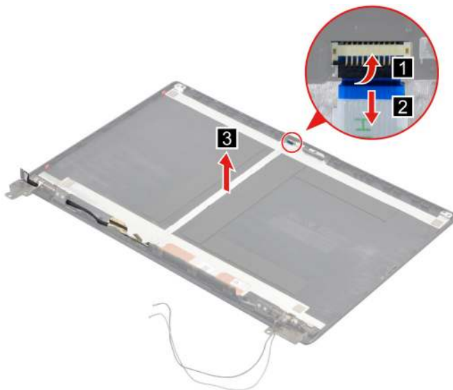
Figure 39. Disconnect the EDP cable from the camera board and then remove the EDP cable
