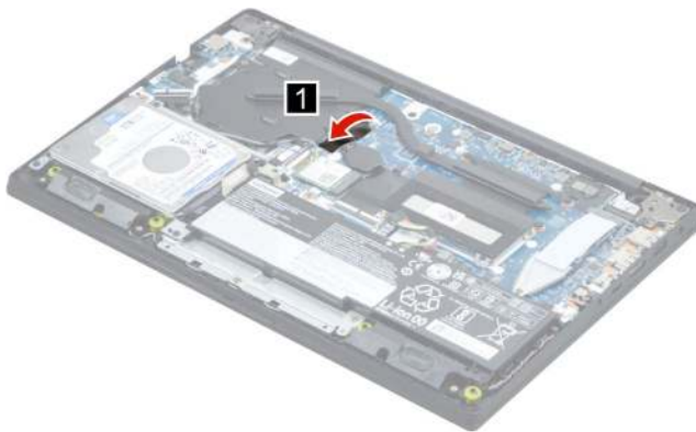
Figure 17. Peel off the motherboard mylar
