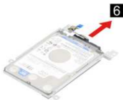
Figure 9. Remove the HDD cable
