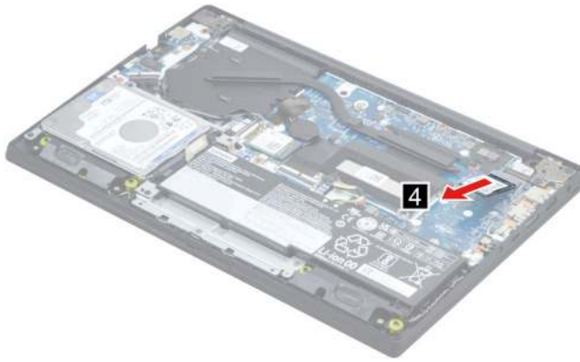
Figure 15. Remove the SSD by pulling it away from the slot
