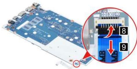
Figure 66. Disconnect the touchpad board cable from the system board
