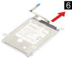
Figure 42. Remove the HDD cable
