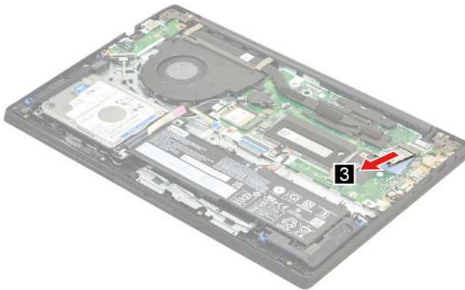
Figure 47. Remove the SSD by pulling it away from the slot
