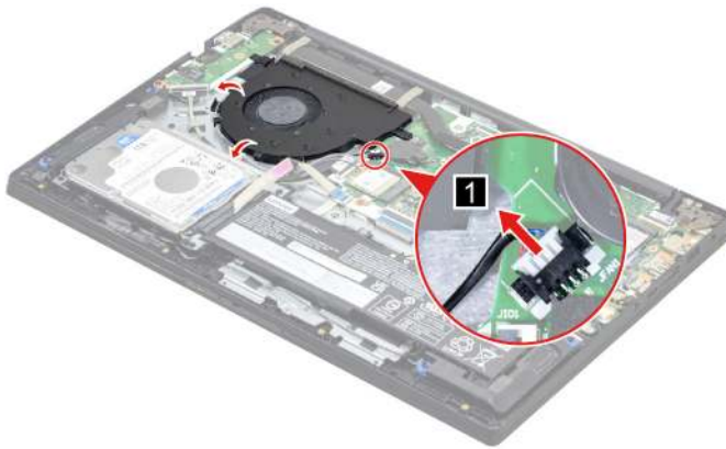
Figure 54. Disconnect the fan cable from the system board
