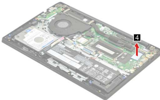
Figure 48. Remove the SSD thermal pad
