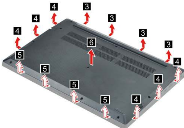
Figure 39. Pry up the latches and remove the lower case
