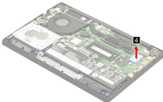
Figure 13. Remove the SSD thermal pad
