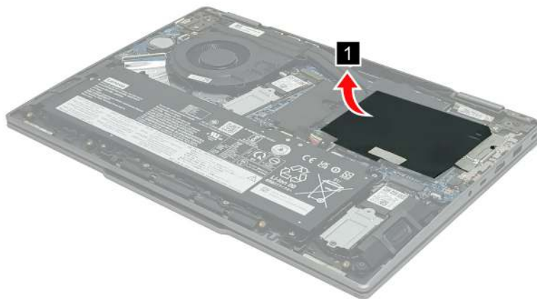
Figure 16. Remove the foil mylar from the memory module
