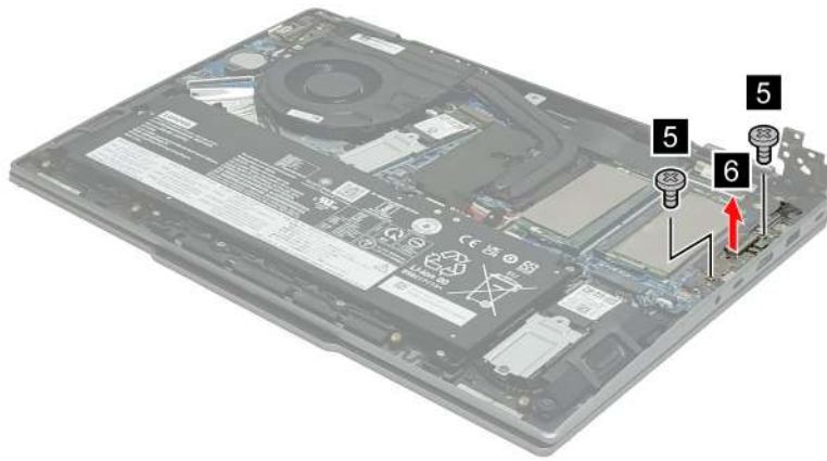
Figure 22. Remove the I/O bracket
