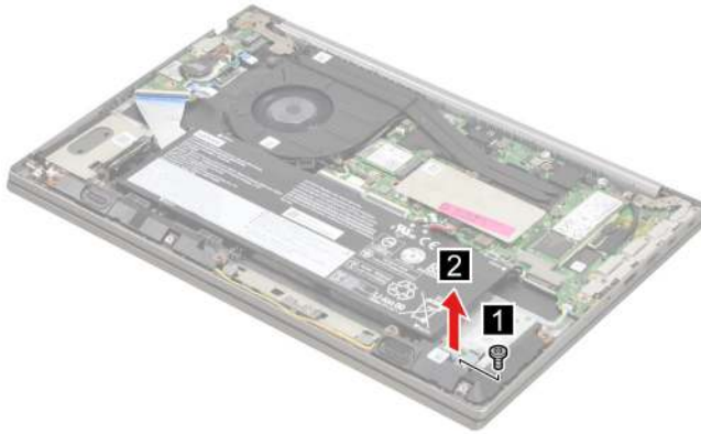
Figure 55. Remove one screw and remove the 2 nd SSD bracket
