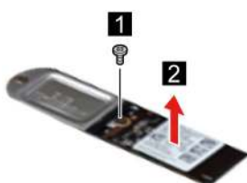
Figure 8. Remove one screw and separate the 2242 SSD from the SSD bracket
