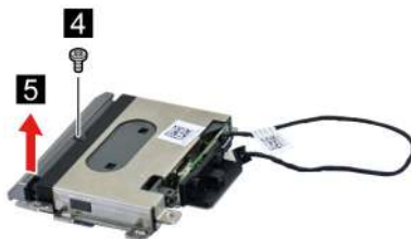
Figure 77. Remove one screw and then remove the ear phone panel
