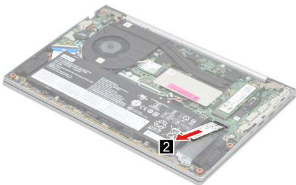
Figure 12. Remove the 2 nd SSD by pulling it away from the slot
