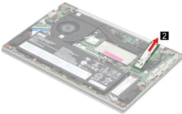
Figure 10. Remove the SSD by pulling it away from the slot
