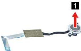
Figure 30. Remove the fingerprint board lens light guide
