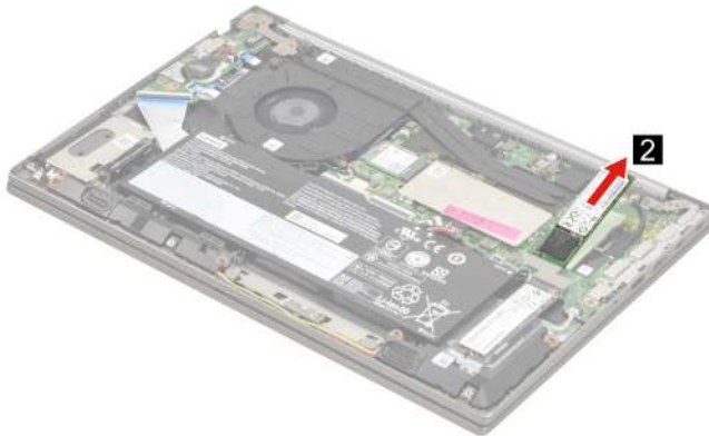
Figure 52. Remove the SSD by pulling it away from the slot
