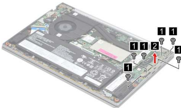
Figure 22. Remove six screws and then remove the I/O bracket (left)
