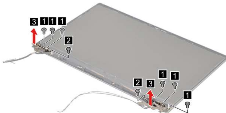
Figure 92. Remove eight screws and remove the hinges
