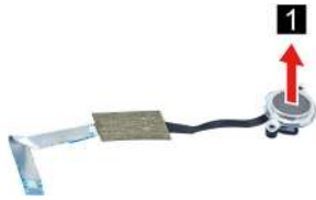
Figure 73. Remove the fingerprint board lens light guide
