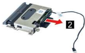
Figure 80. Remove the Bluetooth board module
