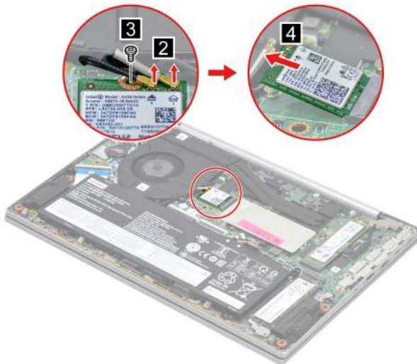
Figure 16. Remove one screw and remove the Wi-Fi card by pulling it away from the slot
