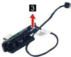
Figure 81. Remove the ear phone Bluetooth board cable
