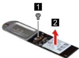
Figure 50. Remove one screw and separate the 2242 SSD from the SSD bracket
