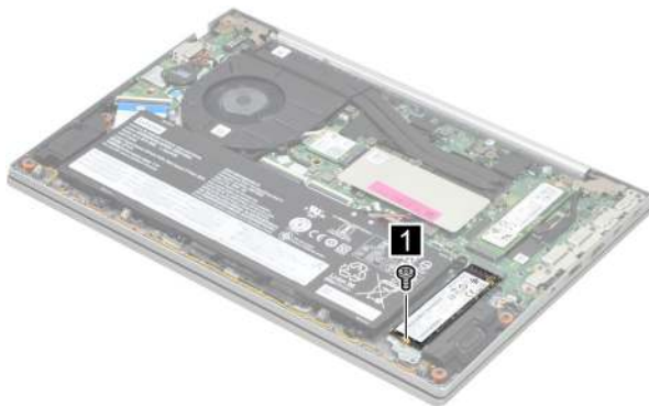
Figure 12. Remove one screw
