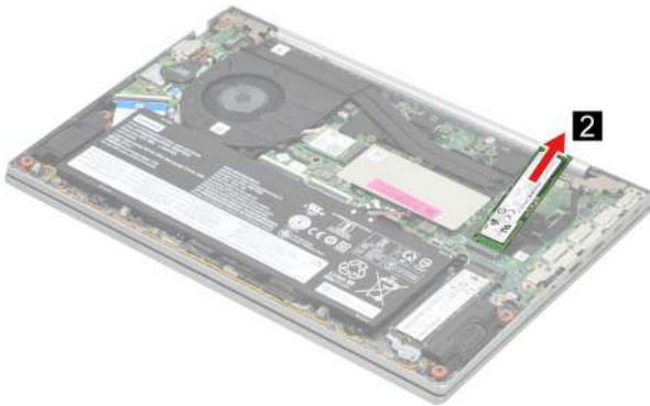
Figure 10. Remove the SSD
