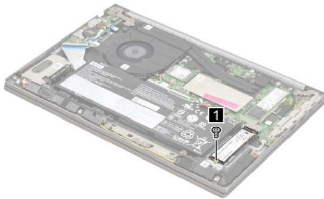
Figure 55. Remove one screw
