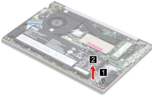
Figure 14. Remove the 2 nd SSD bracket
