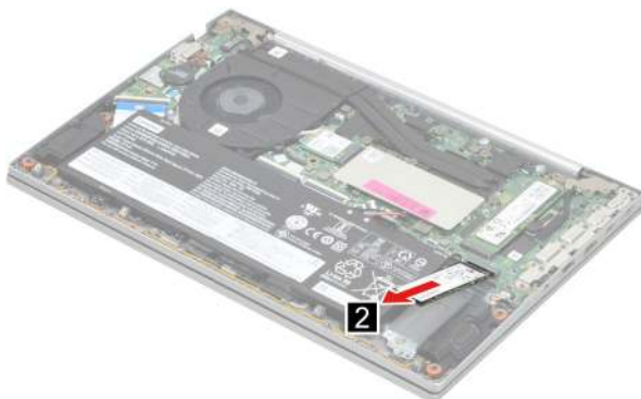
Figure 13. Remove the 2 nd SSD
