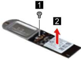
Figure 52. Remove one screw and separate the 2242 SSD
