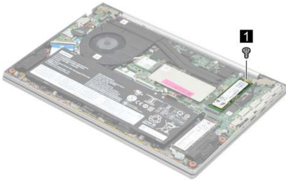
Figure 9. Remove one screw
