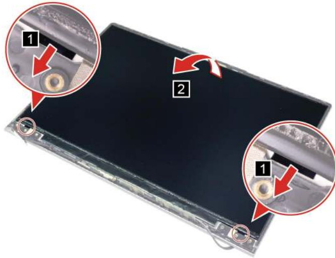
Figure 42. Pull out the adhesive tapes lift up the LCD panel
