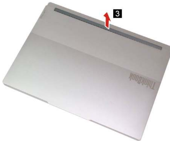
Figure 43. Remove the hinge cap
