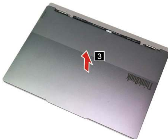
Figure 45. Remove the LCD module
