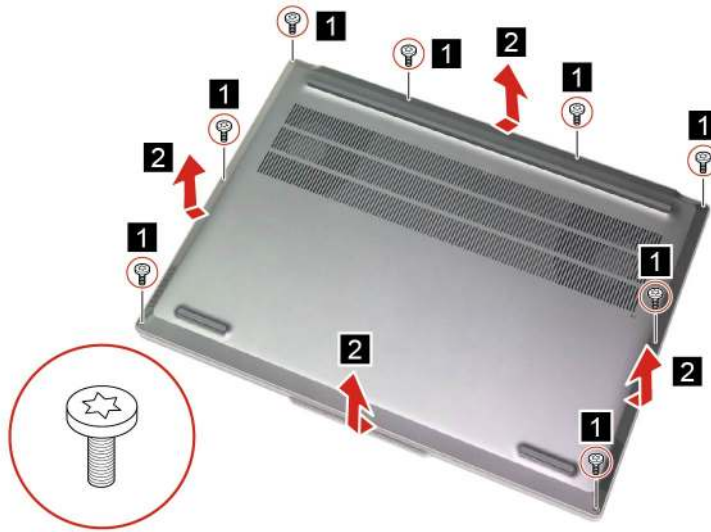
Figure 5. Remove eight screws and the lower case
