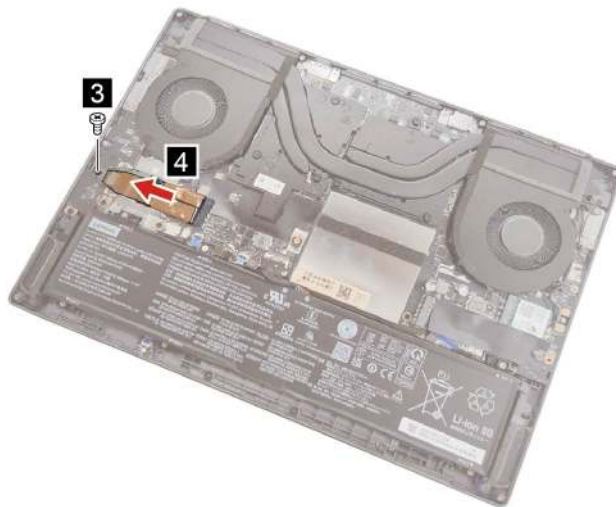
Figure 13. Remove one screw and the 2242 SSD module
