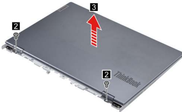
Figure 40. Lift the LCD module
