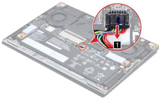
Figure 5. Disconnect the battery pack cable.
