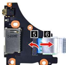
Figure 22. Separate the USB board cable from the USB board
