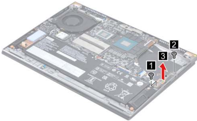
Figure 19. Remove the SSD bracket
