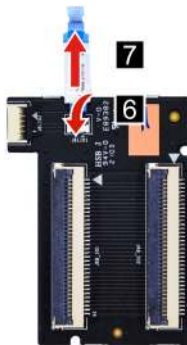
Figure 35. Separate the keyboard backlight cable from the connector board
