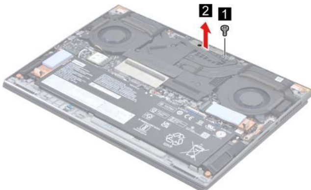
Figure 13. Remove the DC-in bracket.
