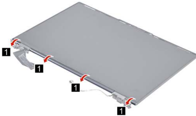
Figure 43. Remove the hinge cover
