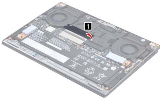
Figure 14. Peel off the memory module mylar
