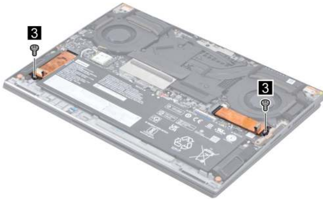
Figure 7. Remove two screws
