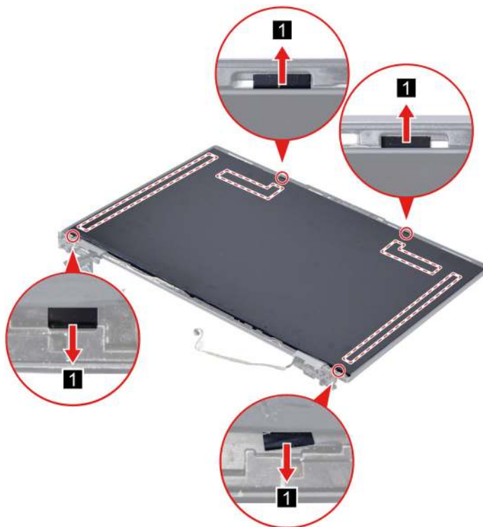
Figure 44. Remove the four pieces of removable tape with tweezers
