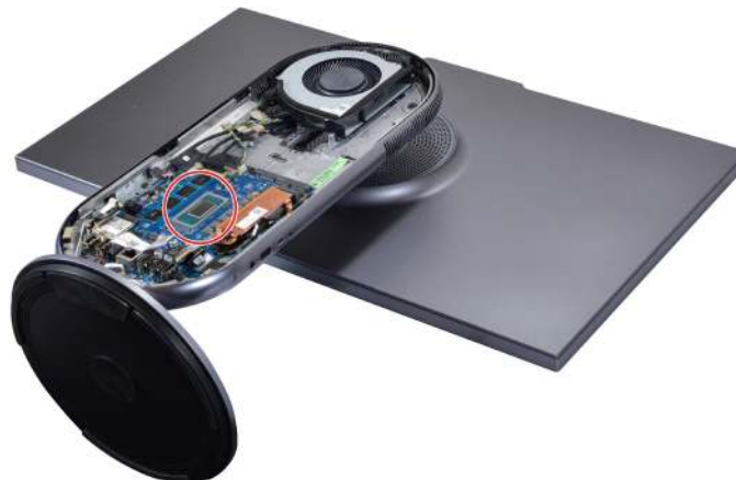
Figure 2. Processor surface area requiring TIM removal prior to reinstallation
