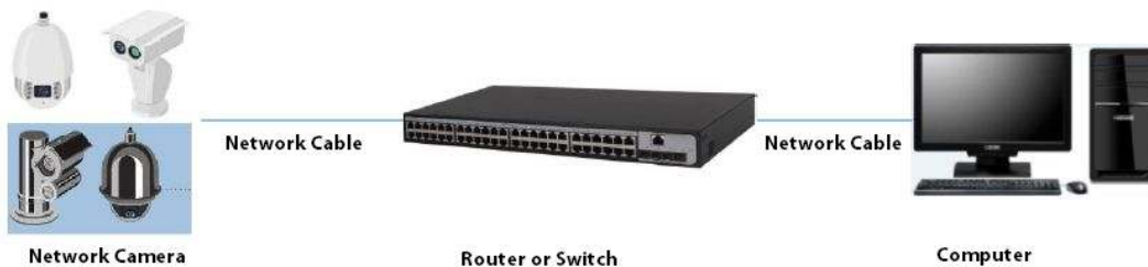
Figure 1-2 Connected through network router or switch
