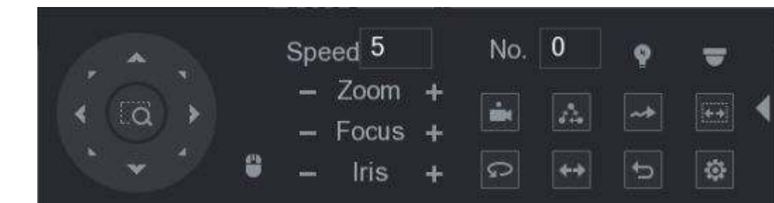
Figure 5-62 Expanded PTZ control panel
