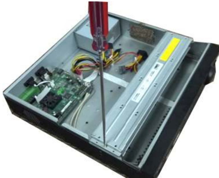
Figure 3-37 Open the top cover
