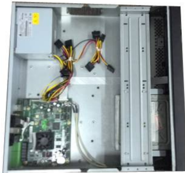
Figure 3-45 Put bracket back
