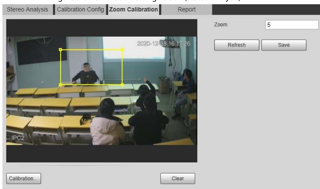
Figure 5-81 Calibration configuration (stereo analysis)
