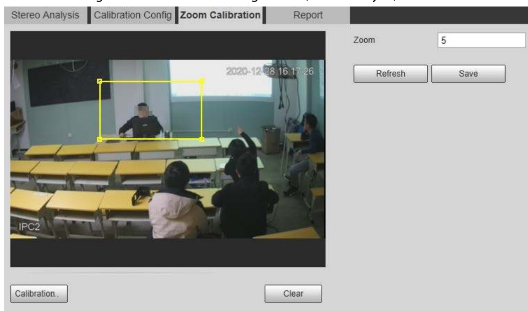
Figure 5-81 Calibration configuration (stereo analysis)
